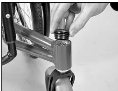
Image 43 Remove the bearing housing cap
